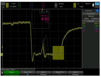
Figure 12. Hardware InfiniiScan Zone triggers immediately.
