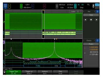
Figure 37b. Gated FFT time correlating the FSK frequency hopping with an I²C command (write 7 @ 0x71 data 10).
