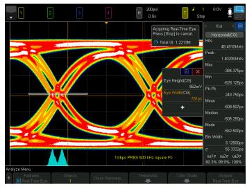
Figure 21. A real-time eye diagram measurement of a jittery 1-Gbps PRBS embedded clock signal. The histogram indicates a bimodal distribution and measured about 55-ps rms jitter.
