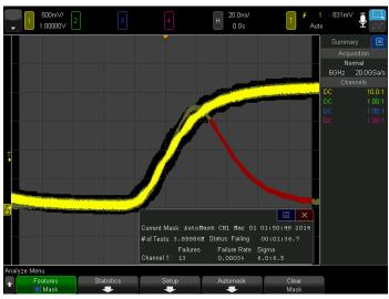
Figure 40. Limit testing of infrequent glitch.
