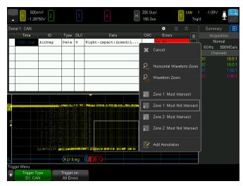
Figure 13. Setting up the InfiniiScan Zone trigger in addition to a CAN bus error packet trigger.
