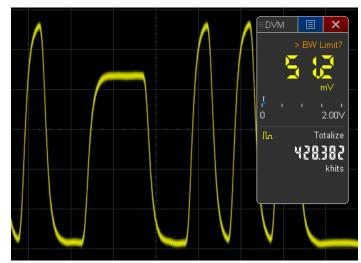
Figure 35. Totalizing the number of runt errors.
