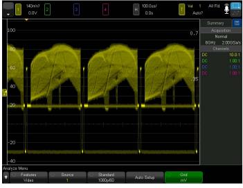
Figure 45. Triggering on a 1080p/60 signal.
