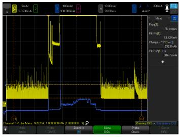
Figure 57. Capturing both zoom out and zoom in view of a cell phone's current consumption inside and outside of its sleep state.
