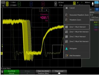
Figure 11. Draw a zone (box) around the anomaly.
