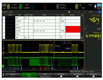
Figure 30. USB 2.0 protocol trigger and decode option display.
