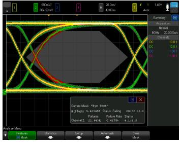
Figure 41. Mask testing of serial data.
